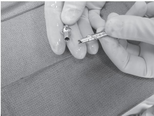
**FIGURE 3** Broken reamers during harvest.
